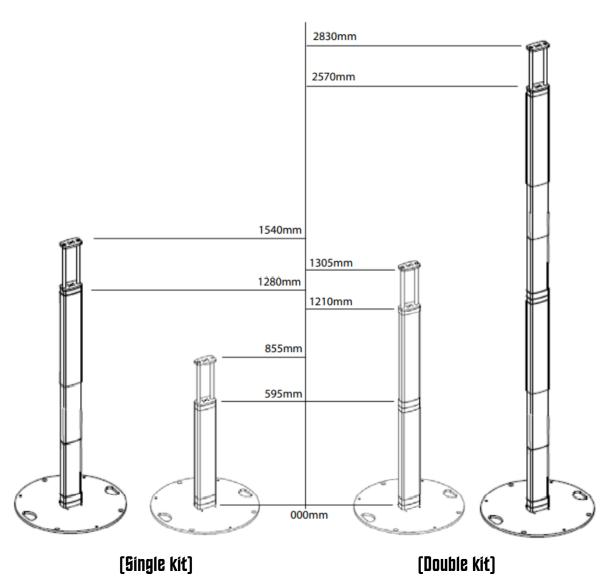
on optional Heavy Duty base Single system stowed and extended
