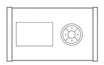
In any menu, push and hold the **Ok** button for 2 seconds and it takes you to the status screen and quick access to the Up/ Down facility.
