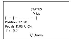
In any menu, you can press and hold the  ${\bf Ok}$  button for two seconds and you will be taken directly to the status screen.
